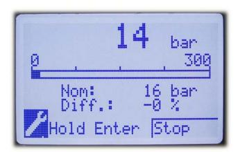
The upper part of the display shows the output pressure of the controller in bar.
