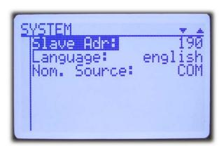
Within **System**, the setpoint source is selected. If **COM** is set, the setpoint is only set via the communication interface. The slave address as well as the language can be selected.
