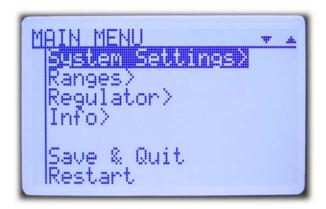
By pressing the **ENTER** key for approx. 3 seconds, the main menu opens. The arrow keys are used to navigate and change the values. Confirm changes with **ENTER**.
