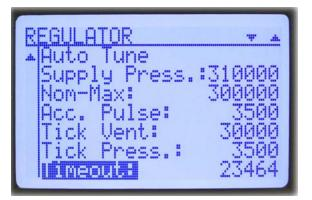
The control parameters P/I/D can be changed in this window.
