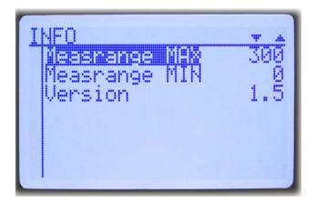
The info area displays the maximum and minimum control ranges as well as the current software version.
